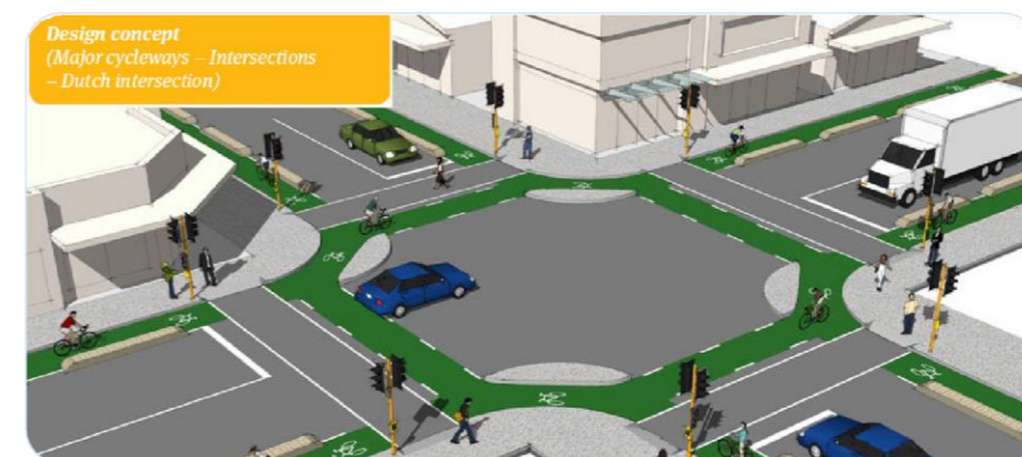
Figure 16: Key Infrastructure Elements of Protected Junction
